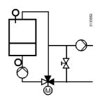
Maintained boiler return temperature controlled via mixing valve
