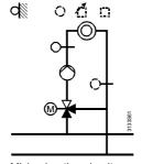
Mixing heating circuit
