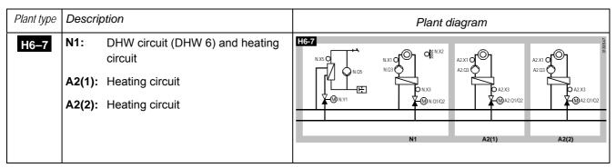
N. Connection terminals of heating controller N1, RMH760B
